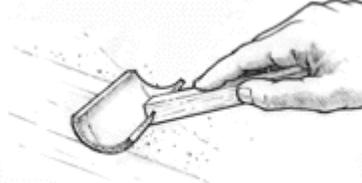
Tip off the coating by dragging a foam roller brush lightly over the fresh epoxy.
