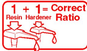
*Pump one full pump stroke of resin for each one full pump stroke of hardener. Depress each pump head fully and allow the head to come completely back to the top before beginning the next stroke. Partial strokes will give the wrong ratio. Read the pump instructions before using pumps.*
