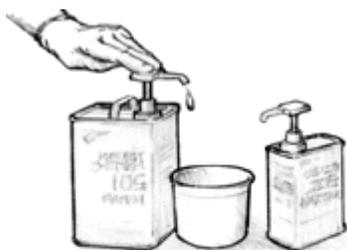
**Figure 2** Dispense the proper proportion of resin and hardener.
